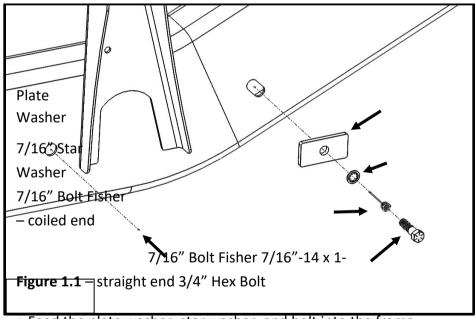
Feed the plate washer, star washer, and bolt into the frame separately, then gently pull on the straight end of the bolt fisher until the threads of the bolt protrude out of the round hole in the frame. Leave the bolt fisher attached.
