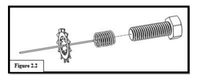
• Pull the non-coiled end of the bolt fisher until the threads of the bolt protrude from hole C. Remove the 1/2" Bolt Fisher.
