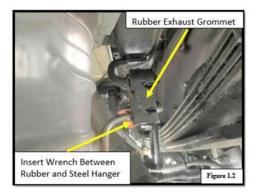
Use a large wrench to adjust the exhaust hanger down to allow for better clearance, Adjust the hanger upward approximately 1/2"-3/4". (See Figure 1.3).
